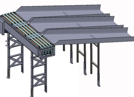
Group of three expulsion device each device can make the expulsion on left or right or both sides
